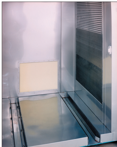
The tracks in the floor indicate that the interior pictured at left is a cart-based system. Also, the hole pattern in the side wall is characteristic of Envirotronics' high-velocity horizontal air flow system.
