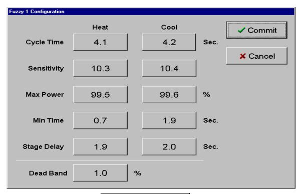
This is the Fuzzy Setup screen used to adjust how the Fuzzy routines are to analyze and respond to received data.
