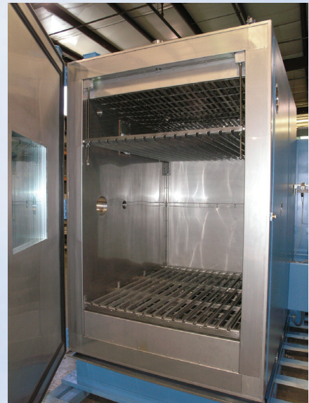
The PVH chamber pictured above features a Vertical Airflow system and Envirotronics' adjustable specimen rack.
