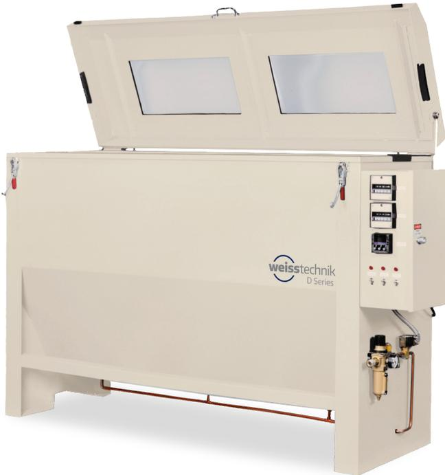
The Weiss Technik D Series Dust Chamber is designed to test a component's resistance to a dust-filled environment as defined in SAE Dust Test Specification J-575, subparagraph "G". The product is placed on the specimen rack and dust is agitated throughout the chamber by injecting compressed air into each of the dust troughs. The dust then settles, covering the product under test.
