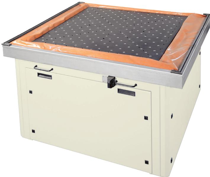
The STAR Series vibration table uses a patented hammer design to provide quasi-random, six degree-of-freedom vibration. A benefit of the STAR Series is the table uniformity, which allows multiple products being tested to receive almost identical forces. The table can be used with the EV Series chamber or separately. The pneumatic air glide system makes moving the table easy.
