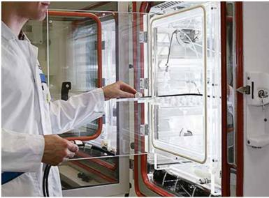
gradients which occur and the associated thermomechanical stresses on the test samples are enormous. One example is a scenario in which vehicle wiring in the floor pan, which has been heated by the engine, is subjected to ice-cold drenching with salt water in winter. In the past, it was only possible to implement these special test requirements manually. With the new air/water temperature shock test chamber, the test is now automated and reproducible, even for large numbers of samples.
