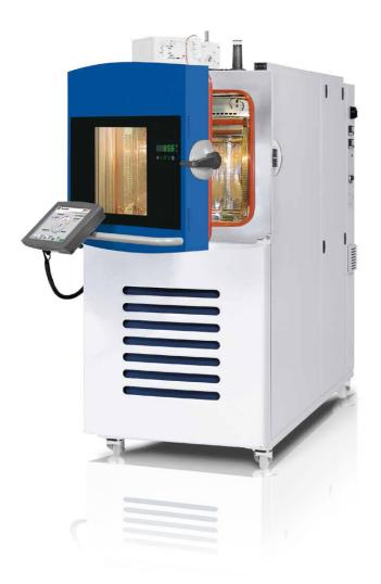
With the **weiss**technik TS temperature shock test chamber, extremely rapid temperature changes ranging from -80 °C to +220 °C can be implemented. The test chamber consists of two independently controlled chambers, one hot and one cold chamber. These are positioned on top of each other. The specimens are placed in a lifting cage and rapidly transferred between hot and cold to achieve a temperature shock. The temperature levels and the number of cycles determine the severity of the test.
