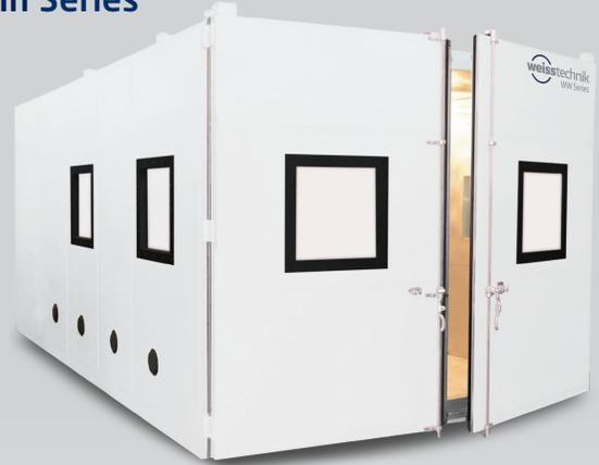
The WW and WP Series of walk-in test chambers offers many pre-engineered and custom solutions that require a larger chamber. Performance features including extended temperature ranges, clear access doors, high floor loading capacity, and more. Temperature range of  $-70^{\circ}\text{C}$  to  $+180^{\circ}\text{C}$  and humidity of up to 98% available.
