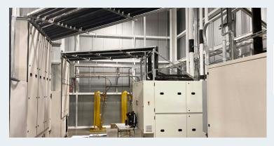
An interconnect system for a Battery Test Center allows for separate chamber and machine pack locations
