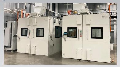
Walk In test chambers are ideal for Battery Pack level testing
