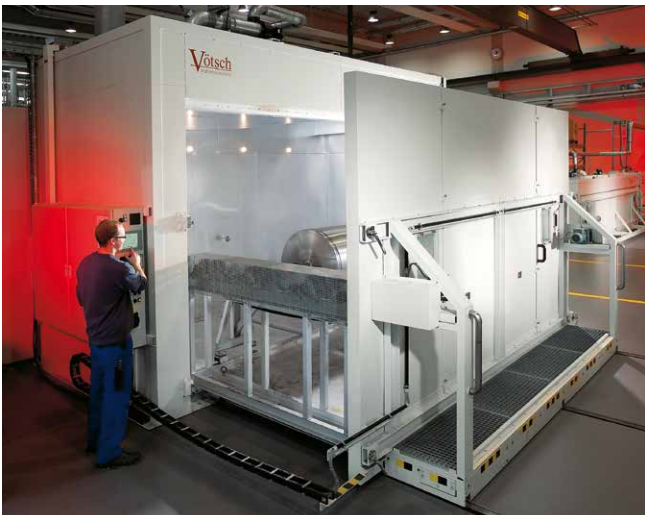
Drawer-type oven with 1 drawer and 1 rotary drive
