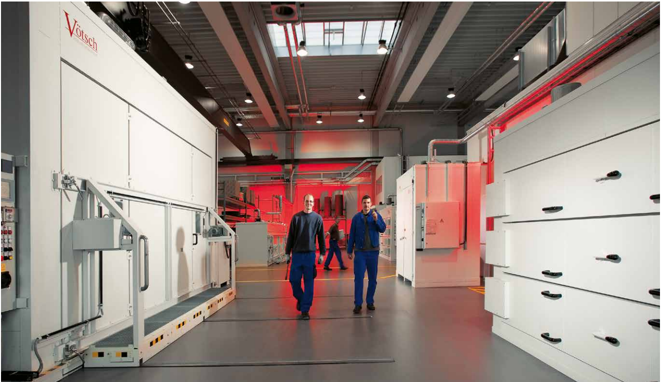
Tempering oven in the CFRP production
