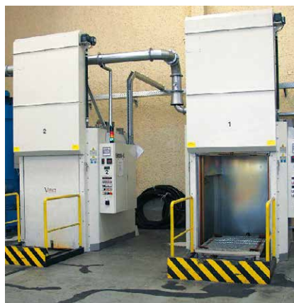
Tempering oven for the automotive industry
