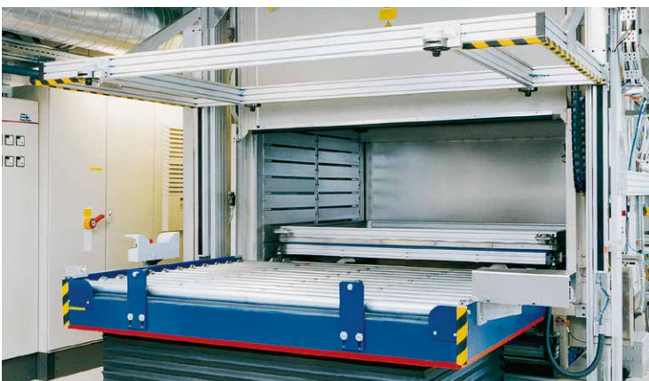
2-zone continuous oven for hardening carbon fibre composite material components in combination with hot air and infrared heating
