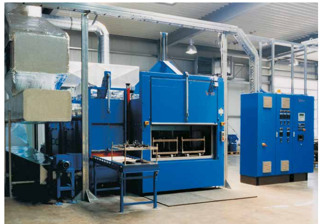
Oven for vulcanization and forming of vehicle coolant pipes
