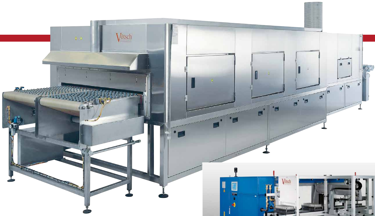
Clean room continuous oven for hardening of sealing plugs used in manufacturing of medicine bottles
