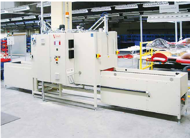
Oven for glue hardening at dashboards
