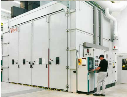
Tempering oven with mobile bogie for use in CFRP helicopter cockpits
