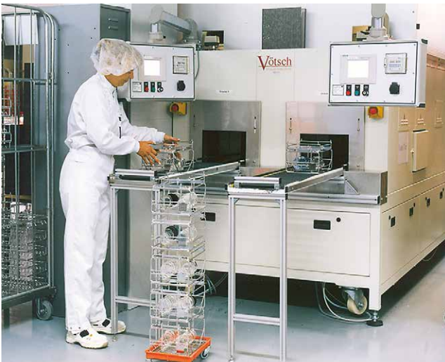
Clean room oven for curing the coatings on plastic glasses
