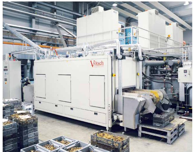
Continuous oven for hardening of sinter metal parts
