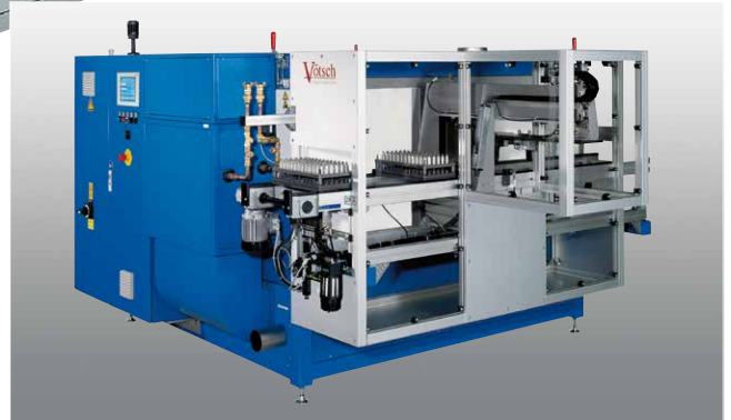
Oven for tempering of compensators
