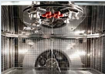
Moveable Product Sensor Measuring of product temperature
