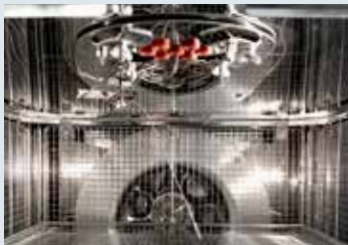
Moveable Product Sensor Measuring of product temperature
