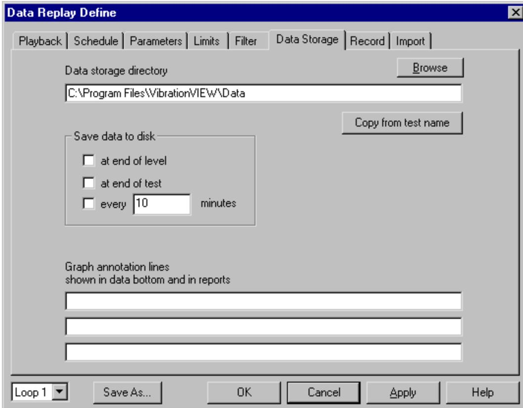
Use this dialog box to set the times at which the test data is automatically saved while the test runs. You can save the data at the end of a level, at the end of a test, or at the end of a time period. All data is saved as a time stamped file that can be viewed at a later time by selecting the File..Open Data menu command.
