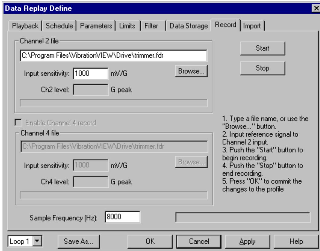
This dialog box is used to record a new playback file from the channel 2 input. Typical use for this dialog box is to connect the output of some playback device (e.g. a DAT recorder) to the Channel 2 input of the VibrationVIEW I/O unit, and then to record this data to the hard drive.
