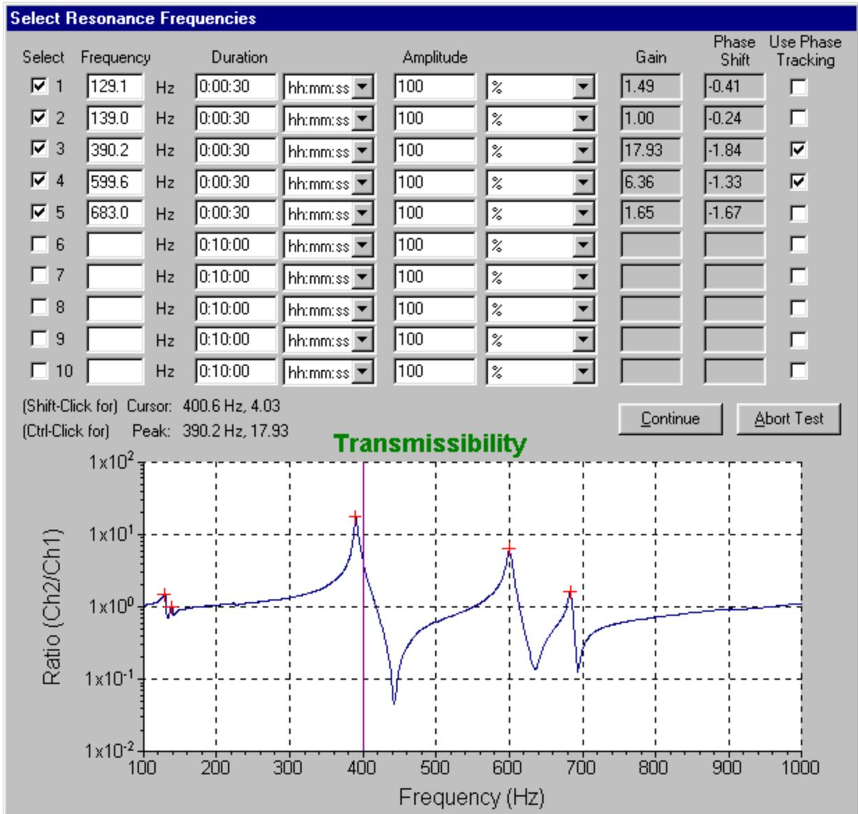
This dialog box appears when a test is running and a "Resonance Table" level is reached in the test schedule. The peaks in the Ch2/Ch1 transmissibility curve are automatically detected and entered into the table. The operator may then select which frequencies to use, or add additional frequencies to the table. When the "Continue" button is clicked, the selected frequencies will be inserted into the test schedule and the test will continue with the first selected frequency.
