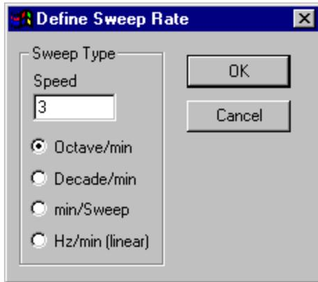
Use this dialog box to set your sweep rate. Enter the rate in the "Speed" box, and click the radio button for the desired units.
