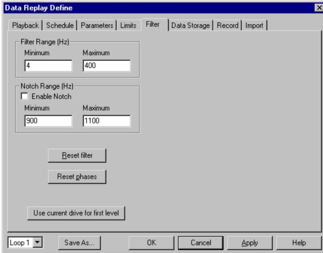
Use this dialog box to display and adjust the filter frequency settings, i.e. to set the frequency range over which the feedback control will operate. You can also enable a notch band to filter out a frequency range in the middle of the spectrum. This is useful for such things as a shake-and-rattle test, where you can see which frequencies are exciting a rattle mode.
