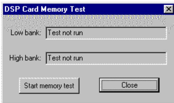
Use this dialog box to verify that the DSP memory is operating properly, and that communication between the PC and the DSP card is working. This command is only available when running in System Check mode. In general, this command only needs to be used if you are instructed to do so by Vibration Research Corporation.
