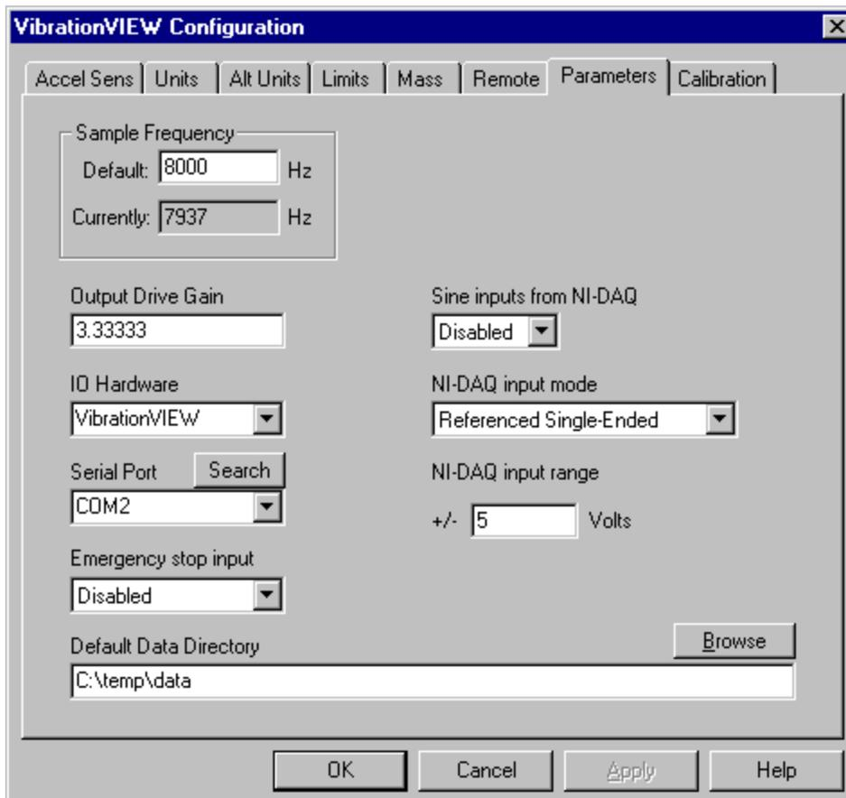
Use this dialog box to set global system parameters including the type of I/O hardware and the serial port used by the controller. This dialog box also may be used to set the default sampling rate, and to see the current sampling rate used by the controller.
