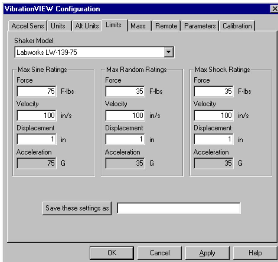
Use this dialog box to configure the limits for your shaker system. These parameters are checked at run time to determine if the test you are about to run is within the specifications of your shaker system. The acceleration and velocity limits are measured 0-to-peak while displacement limits are measured peak-to-peak.
