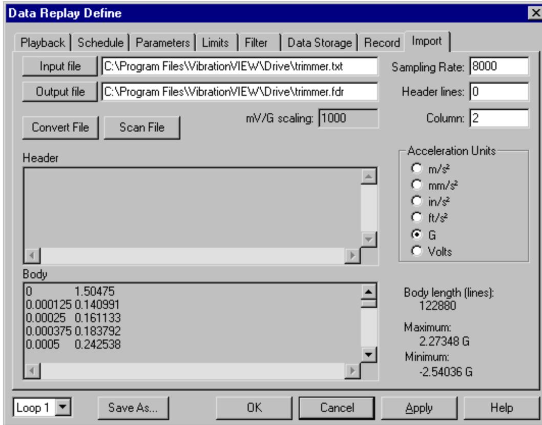
Use this dialog box to import a text file with comma, semicolon, or white space-delimited data into an FDR format file for use as the playback file in Field Data Replicator tests. Select an input file by clicking the "Input file" button. Set the appropriate sampling rate, column number, and acceleration units, and then click the "Convert File" button to convert the file to the VibrationVIEW internal format (FDR format).
