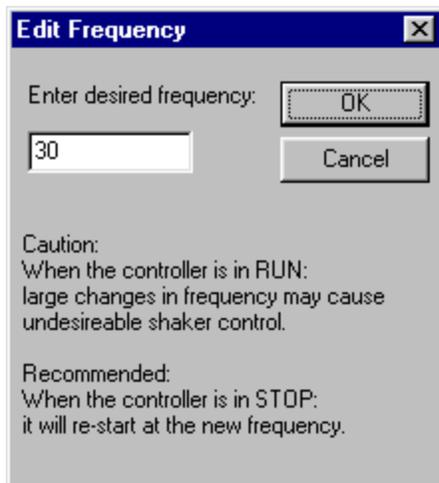
Use this dialog box to set the current and/or the starting frequency in Sine Tests.
