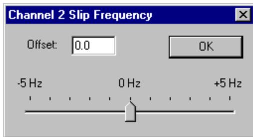
Use this dialog box to adjust the frequency shift for the Constant Output Level Adapter (COLA) output. This is useful for triggering stroboscopes at a frequency slightly shifted from the excitation frequency so that the stroboscope may be used to see device vibration in slow motion.
