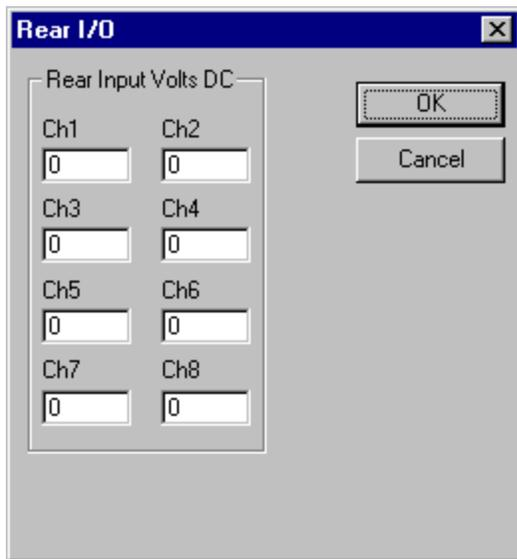
This dialog box is used only for diagnostic purposes. It displays the input values for the 8 discrete inputs on the rear of the VibrationVIEW I/O unit.
