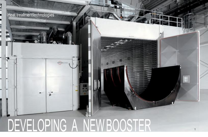
Engineering large CFRP components requires high precision in the heat treatment temperature controls to ensure the finished parts have the correct material properties
