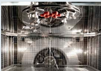
Moveable Product Sensor Measuring of product temperature
