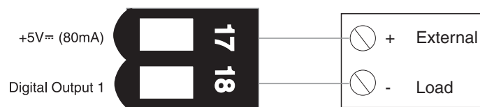
Figure 12.9c — Switched DC Example
